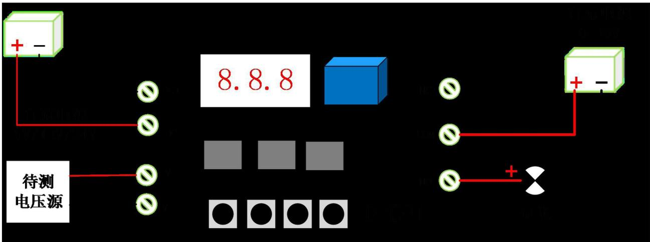
Illustration 1: The first wiring diagram of DVB01
